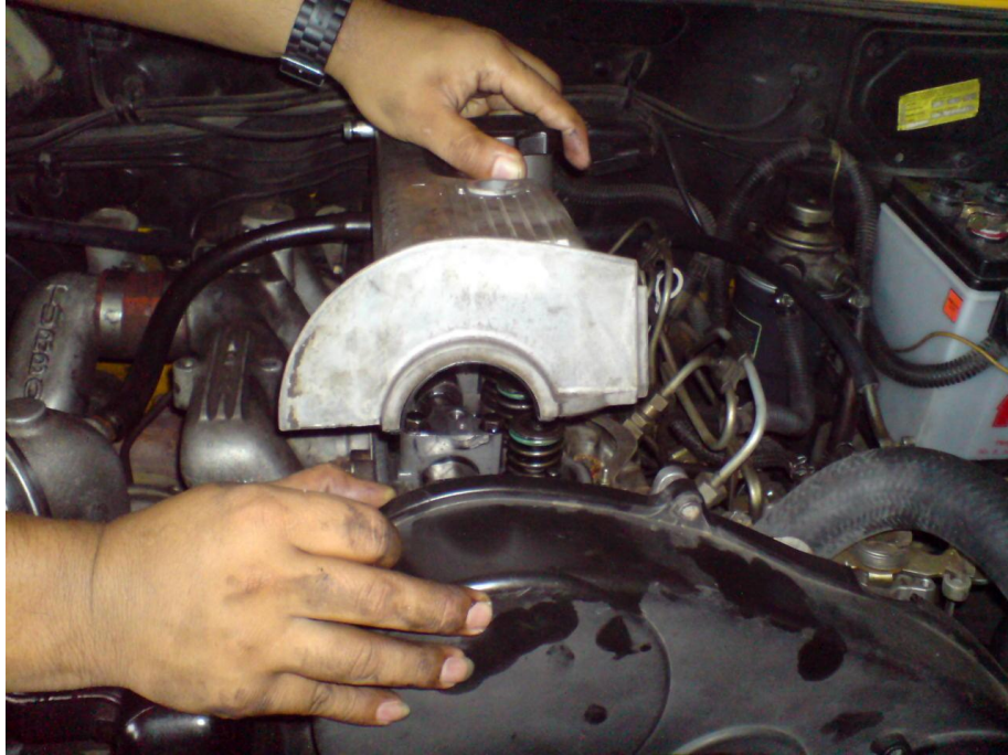
RAJAH 13 : MEMBUKA CYLINDER HEAD COVER
